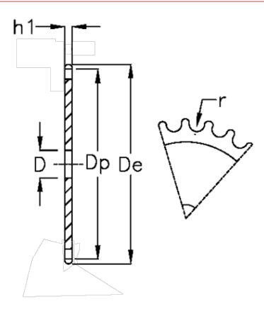
C = 2 D = 14 De = 75 Dp = 67.61 For chain size = 3/4 x 7/16 For chain type = 12 B-1 h1 = 11.1 Sumber of teeth = 11
